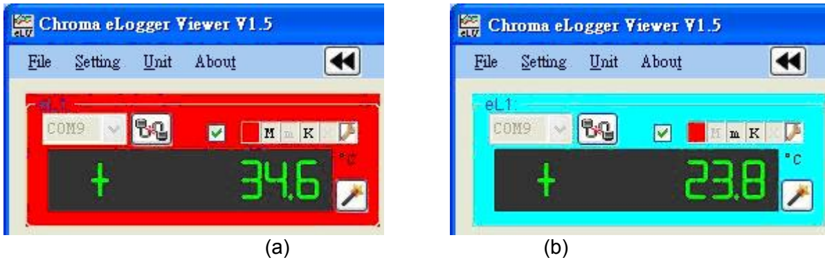
Figure 2-6 Background color in display area changed indicating (a) higher than maximum threshold (red) or (b) lower than minimum threshold (light blue)
